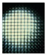
**Figure 8** View through the element of a catalytic converter from a car exhaust. The inner surface is coated with an alloy containing platinum, rhodium and palladium.
