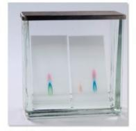
Figure 2 The chromatogram develops on the TLC plate in a tank with the solvent at the bottom. The lid reduces the rate at which the solvent is absorbed and allows for a better separation.
