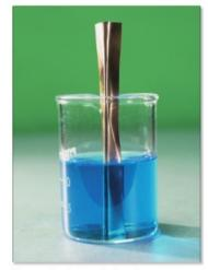
Figure 1 Copper half cell – copper metal is placed in an aqueous solution containing Cu<sup>2+</sup>(aq) ions. An equilibrium is set up at the surface of the solid Cu with aqueous Cu<sup>2+</sup> ions:
