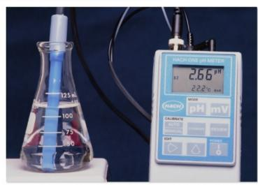
**Figure 2** The pH of a solution of the weak acid methanoic acid is being measured using a pH meter. The concentration of the methanoic acid is 0.030 mol dm<sup>-3</sup> and the pH reading can be seen to be 2.66.
