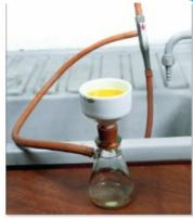
Figure 4 Filtration under reduced pressure.
