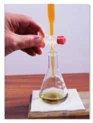
Figure 4 Potassium dichromate titration where this chemical is in the burette.
