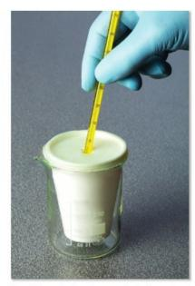
Figure 6 Determining the enthalpy change of solution of potassium chloride, using simple apparatus sometimes known as a coffee cup calorimeter.
