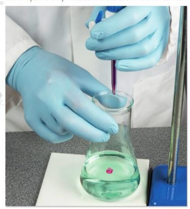
Figure 2 Measuring the concentration of iron(II) ions in a solution of iron(II) sulfate. You can see the purple colour forming as the MnO<sub>4</sub> runs into the acidified Fe2+(ag) solution in the conical flask.
