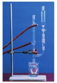
Figure 2 Oxidation of aldehydes is carried out under reflux.
