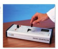
Figure 2 A colorimeter monitors the concentration of a reactant or product by measuring the amount of light passing through a substance.
