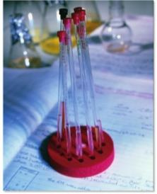
Figure 6 NMR samples are prepared using a deuterated solvent and a tiny amount of TMS. Both the solvent and TMS can be evaporated off after the analysis and this recovers the original sample. Sample recovery is only done if the yield of product was very small or further analysis is required.
