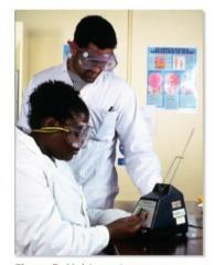
Figure 5 Melting point apparatus.
