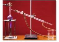
Figure 2 Quickfit apparatus for distillation.
