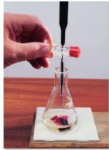
**Figure 2** Measuring the concentration of iron(II) ions in a solution of iron(II) sulfate. You can see the purple colour of the  $MnO_4^-$  before it reacts with the acidified  $Fe^{2+}(aq)$  solution in the conical flask.
