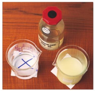
**Figure 1** The reaction between sodium thiosulfate and hydrochloric acid is an example of a clock reaction. The time taken for the precipitate formed to obscure the cross is measured at varying reactant concentrations.  $\frac{1}{t}$  is then used as a good approximation of the initial rate for each set of concentrations.
